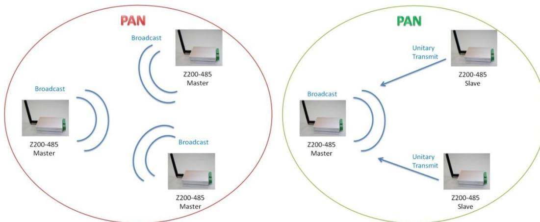
When a Master mode FBs-CMZBR sends RF packets, it broadcasts the packet to all the devices with the same PAN ID. On the other hand, when a FBs-CMZBR, as a Slave, sends data wirelessly, it only sends the data to the Master with a same PAN ID. In order for a Slave to work with a Master, user must pair each other. After successful pairing, the Slave will remember the Master' s address and will be able to send RF packet directly to the Master.
