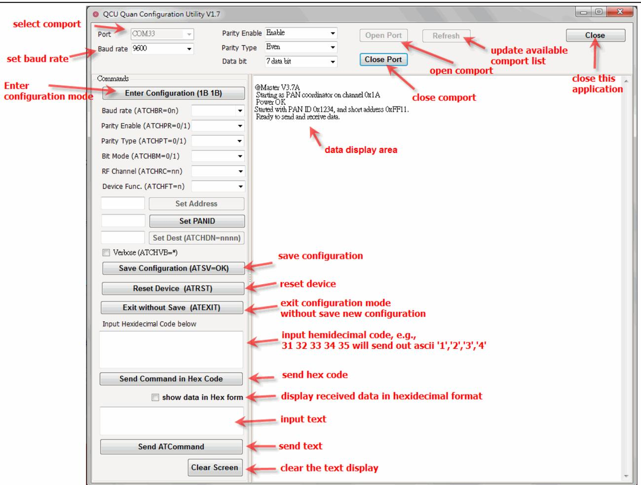
iii. In QCU, choose the correct COM PORT number and press "Open Port" button. Then the QCU is able to talk with the connected FBs-CMZBR.
